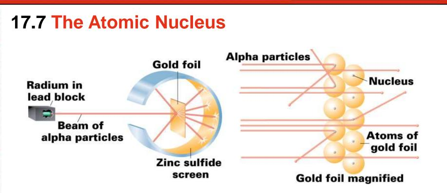
The occasional large-angle scattering of alpha particles from the gold atoms led Rutherford to the discovery of the small, very massive nuclei at their centers.
